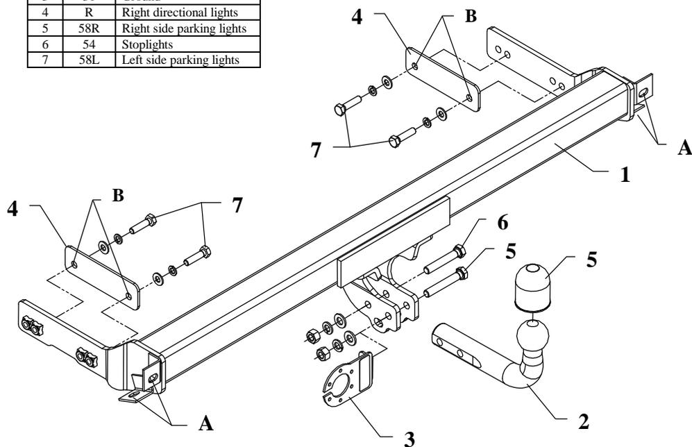
This towbar is designed to assembly in following cars: **VOLKSWAGEN PASSAT CL version 2**, produced since 04.1988 till 09.1993, catalogue no. **K010** and is prepared to tow trailers max total weight **2000 kg** and max vertical load **75 kg**.
